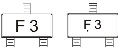
Solid dot = Green molding compound device, if none, the normal device.
